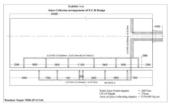
In RSMT Juice collection system of vacuum filter, there are 6 up and 8 down juice collecting nipples each of ID 27 mm. Up and down nipples have separate header of ID27 mm. Upper header of one segment and down header of 2<sup>nd</sup> consecutive segment are connected with main headerof ID41mm at the center of the drum. There are 20 nos. main tube headers. Each tube header is routed to main vacuum filter tube plate header. Juice Collection Arrangement is shown Sketch No. 1-B
